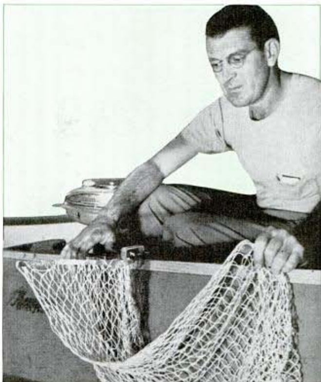
Fish holder built like elongated landing net attached to side of boat for keeping captured fish alive
